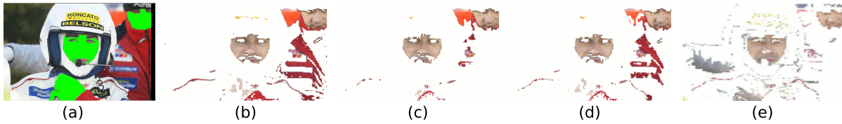
Figure 7: Visual results of detected skin for the three color space algorithms and the texture approach: (a) hand segmented skin, (b) RGB, (c) HSV, (d) YcbCr and (e) SVC texture.
